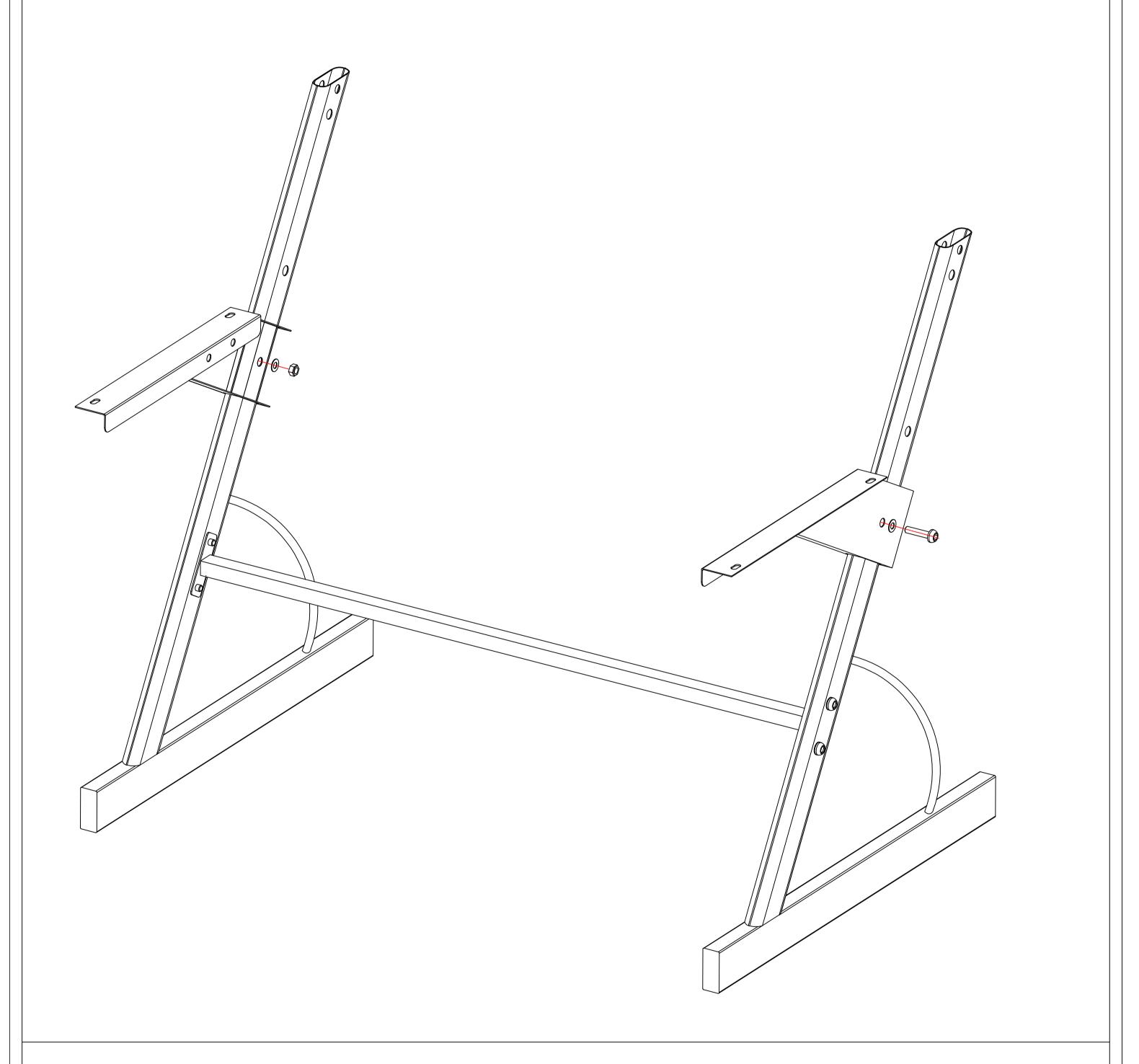
2. Assemble two main shelf supports on to legs as shown and tighten the bolts.
