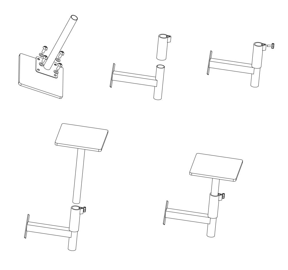
5. Assemble monitor support wings as shown in illustrations.
