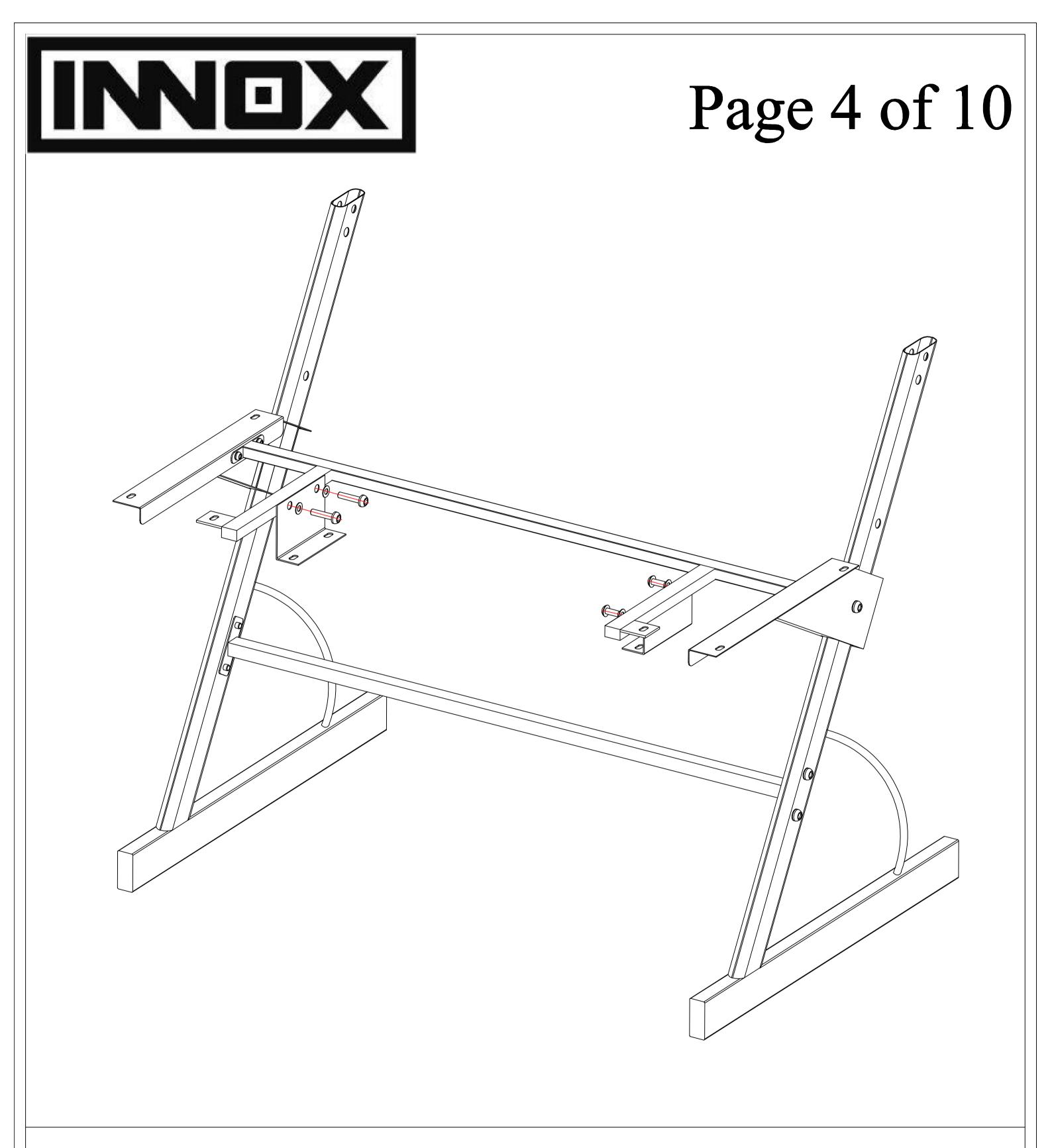
4. Put two keyboard shelf brackets on and tighten the screws as the picture showed.
