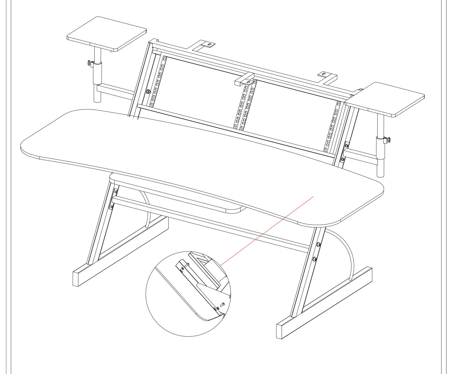
9. Center shelves on support brackets and at desired depth and mount in place with provided wood screws.
