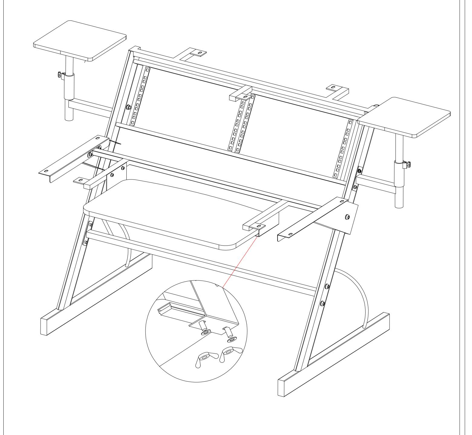
8.Place the keyboard shelf on the keyboard shelf brackets and bolt in place, tightening nuts until desired shelf pull-out tension is achieved.
