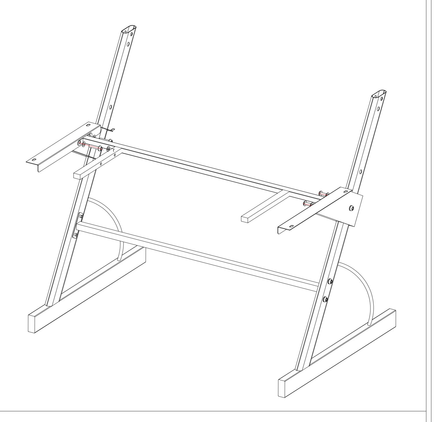
3. Connecting the main shelf cross bracket as the above picture and tighten the screws
