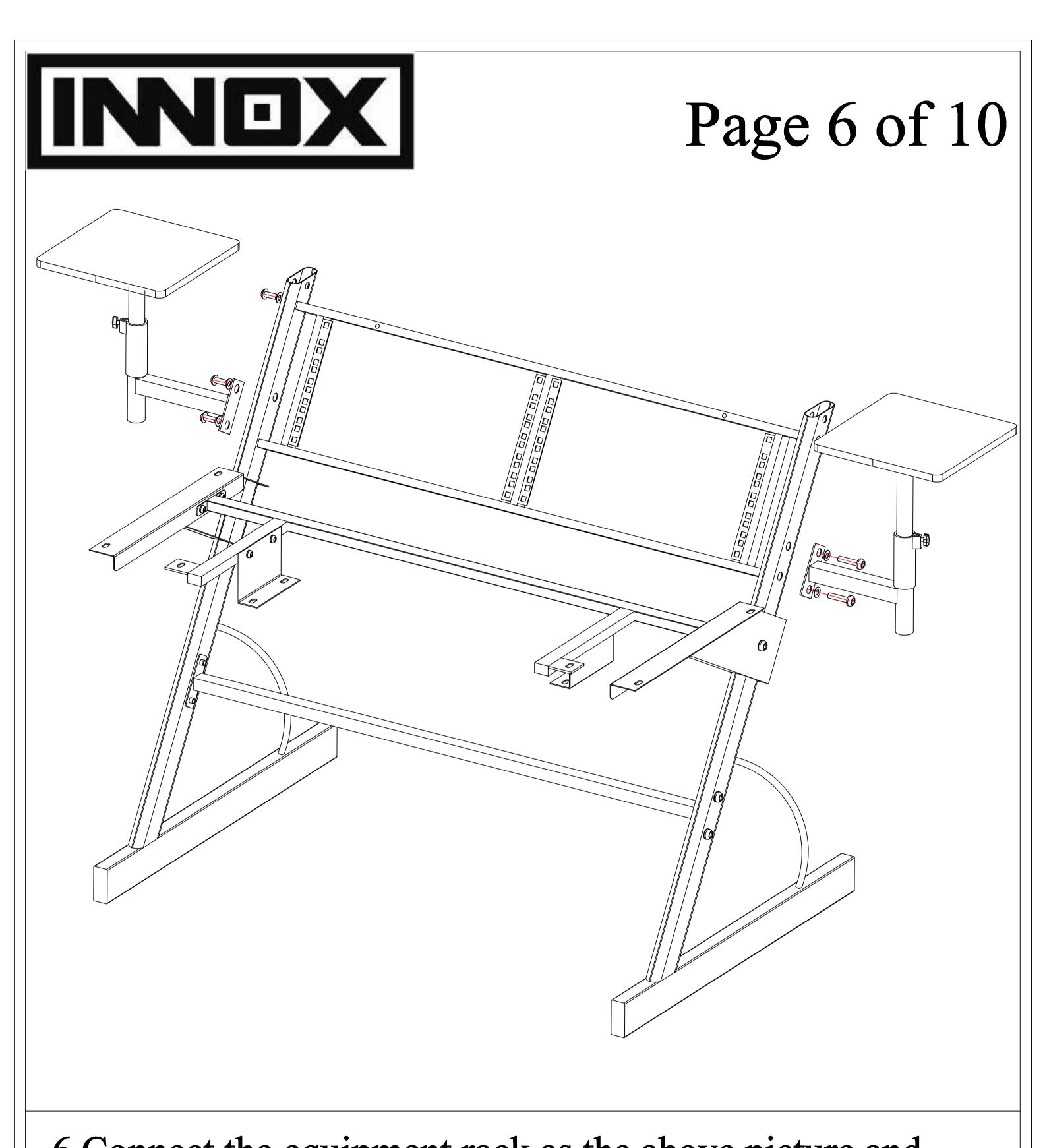
6.Connect the equipment rack as the above picture and tighten the screws, and mount monitor wings on to main desk supports in holes shown and tighten bolts firmly.
