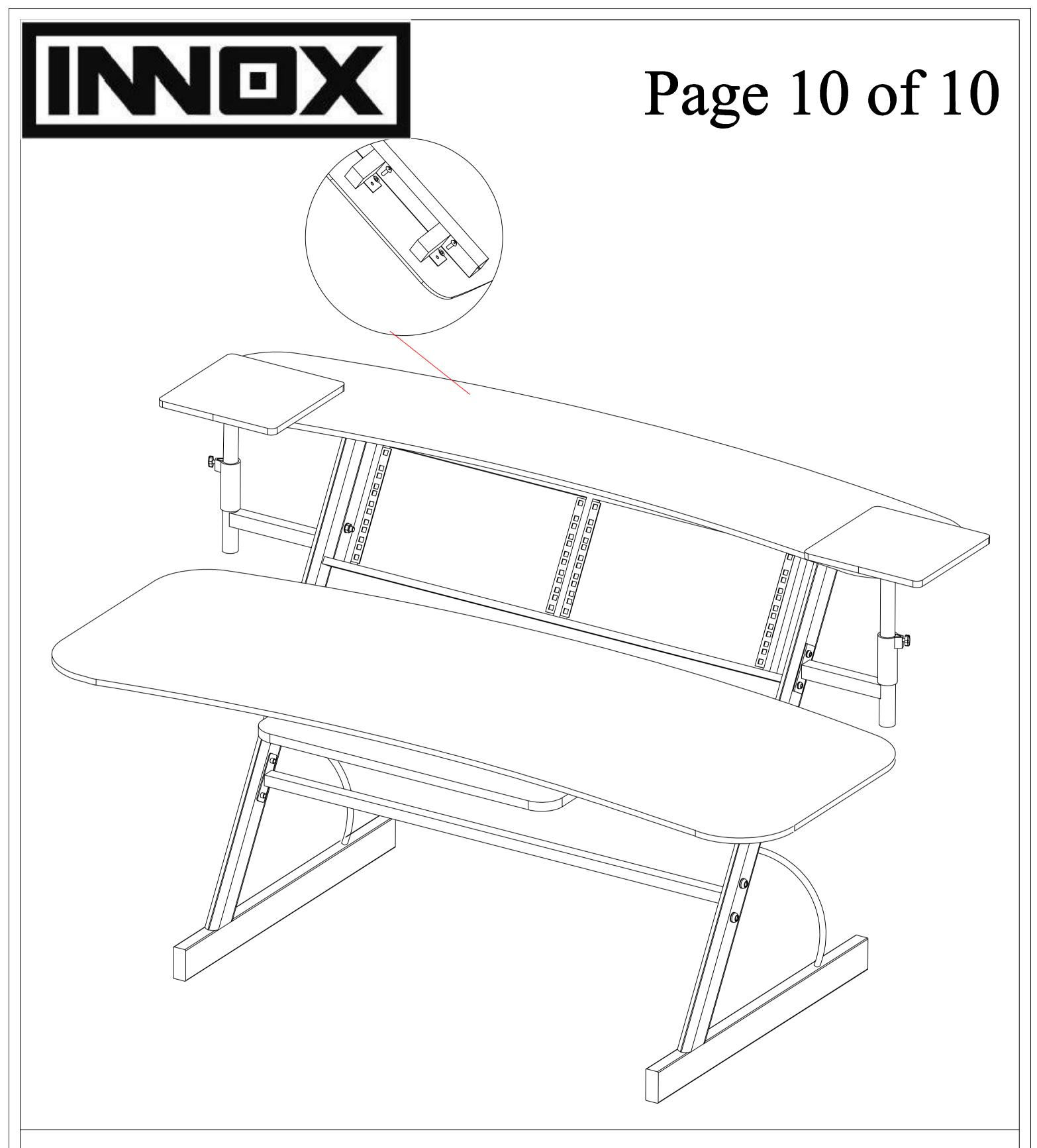
10. Center shelves on support brackets and at desired depth and mount in place with provided wood screws.
