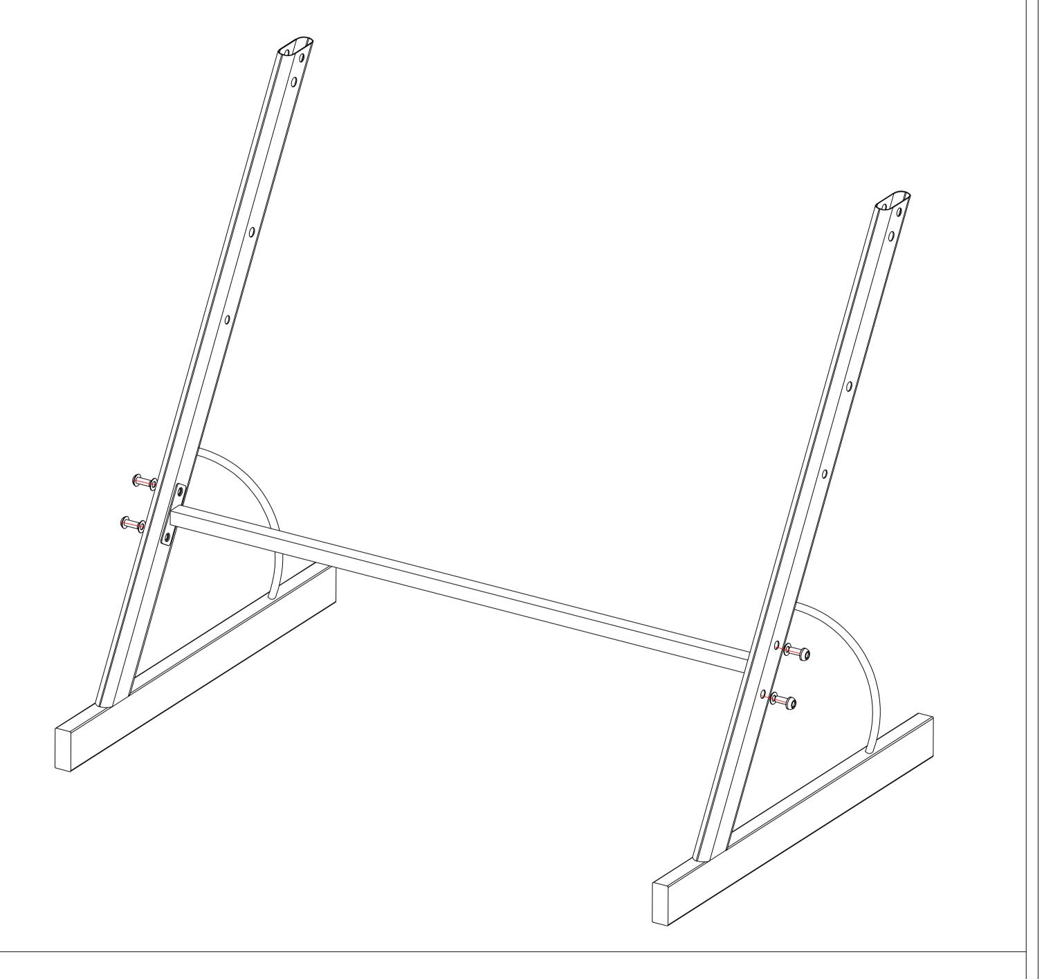
1. Attach two main legs together with bottom cross-support bar.
